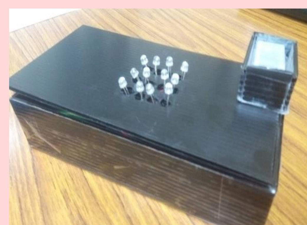
Fig 1. The device with an Arduino to simulate the glycan array mechanism.
